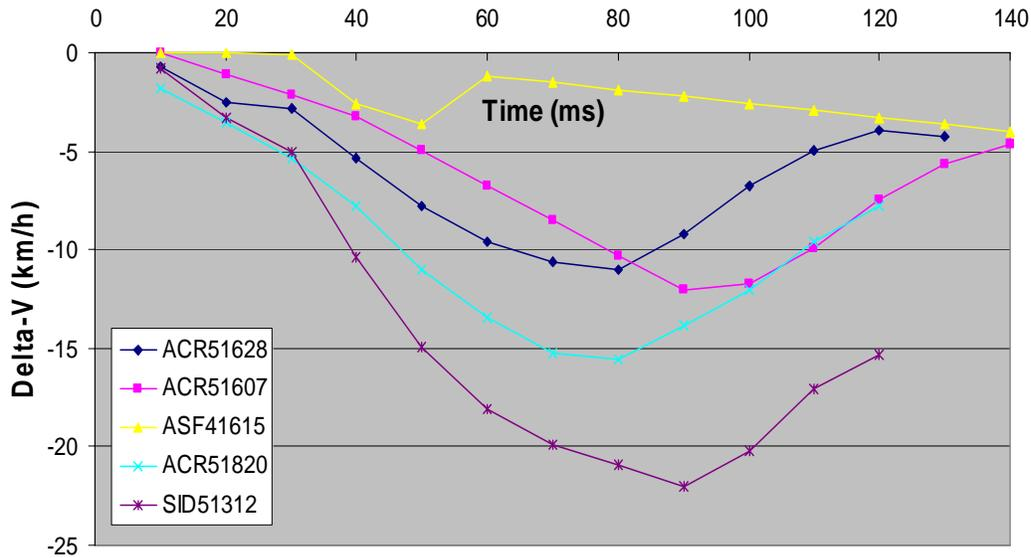
Figure V Cumulative delta-V for cases with acceleration recorded during crash pulse
