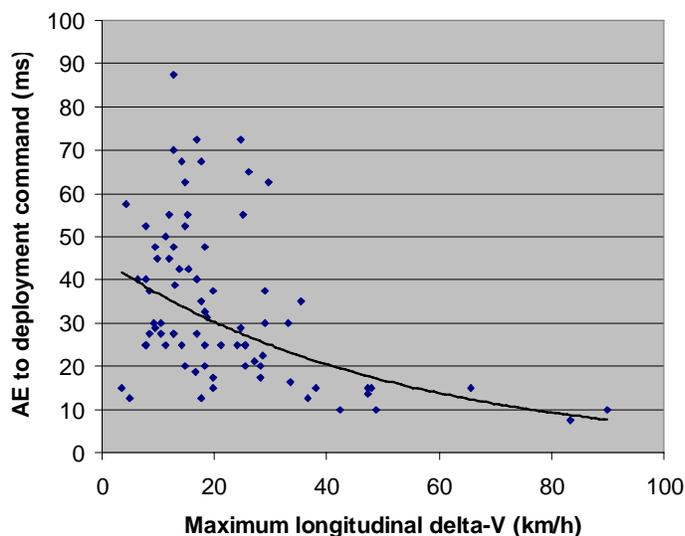
**Figure VII Airbag deployment command timing versus delta-V**
